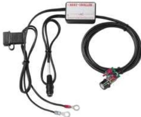
Technical Specifications: Size - 1.5 in x 2.25 in x .85 in or 38 mm x 57 mm x 21.5 mm Switch and LED on PC board on 5ft cord for Panel Mounting .8in L x .9in W x .7in H Comes with Attached 18 inch battery harness with 15 amp fuse. Mounts out of sight providing a clean installation
